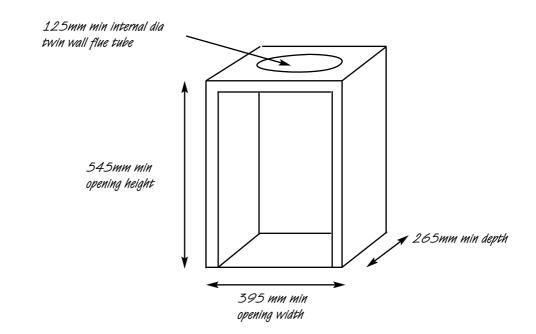
Some flue boxes may require minor adaption when fitting the fire using the cable fixing kit. The firebox, base of the flue box, and the hearth may be drilled to allow plugs and screws to secure installation.
