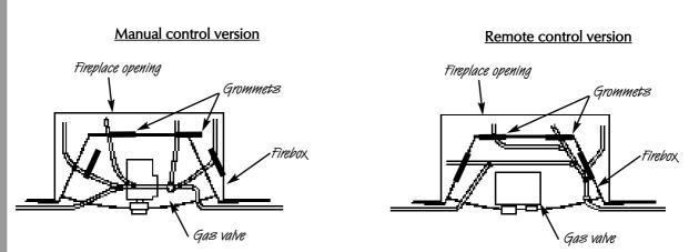
The gas pipe must be suitably protected where it passes through fireplace openings. Any sleeving should be sealed to the pipe at its ends.
