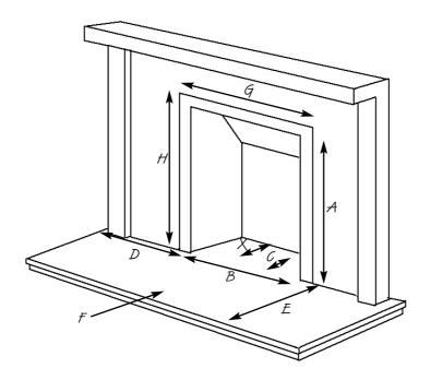
A. Opening height: 545mmmin/575 mm max.B. Opening width: 390mmmin/440mm max.
